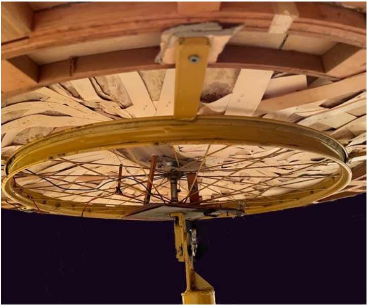
ABOVE: The track is powered from two brass pickups mounted underneath the wheel rubbing on scored copper-clad circuit board attached to the top of the stand. The bolted pairs of pieces of wood hold the pickups. The quarter inch phone jack socket on the left permits an easy electrical connection to the direct current power source.
