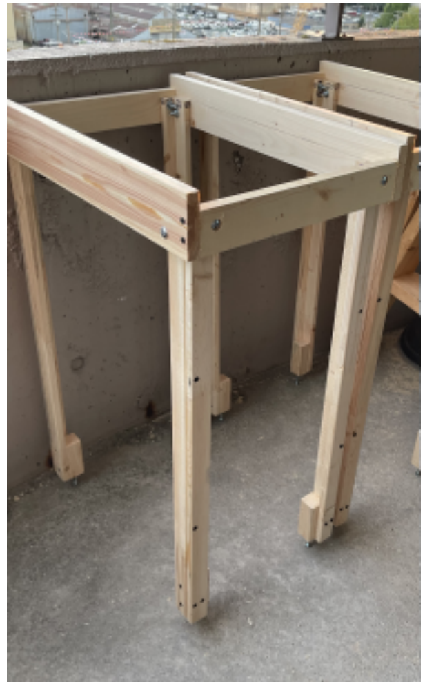
ABOVE: Adaptations were made to the original design by lowering the module ends, allowing the two-foot foam sections to sit flush and connect seamlessly from foam to foam.
